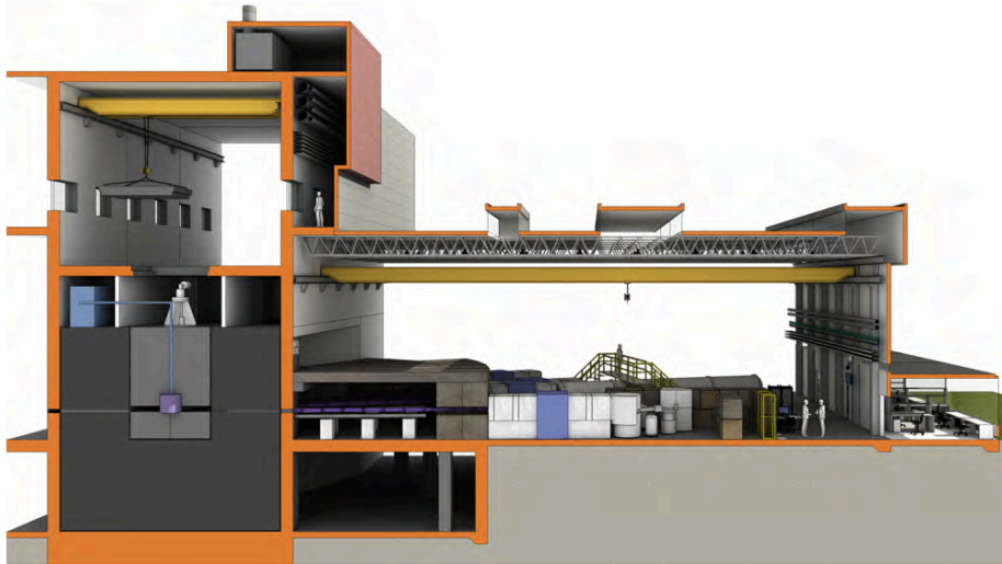
Figure 1: General conceptual layout of the target station. The target monolith is shown at the left, the moderator, premoderator and reflector unit is located in the centre of it. A representative neutron beam line serving a scientific instrument is on the right.
