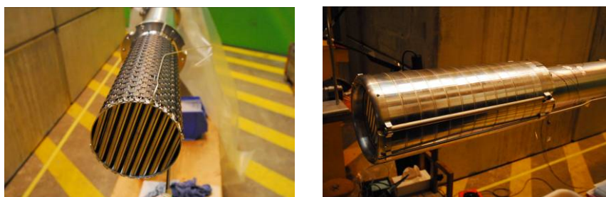
Figure 4: SINQ Target 7, without (left) and with the lead-containing reflector rings (right), ready for getting the safety shroud mounted.
