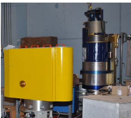
Figure 8: The secondary spectrometer of EIGER in place on the high-precision granite (left) and the lower part of the base monochromator shielding with turning unit.
