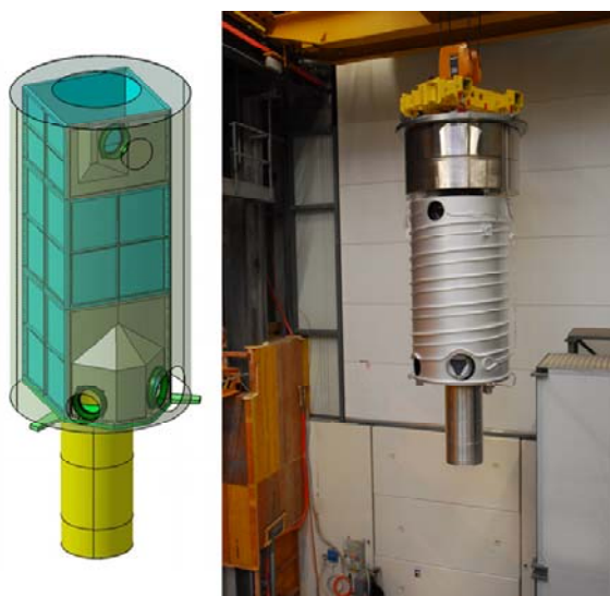
Figure 10: Finished setup of the UCN storage volume surrounded by the heat radiation shield, vertical UCN guide on the bottom and ~10 tons steel shielding on top (about 5m tall): a) design drawing, b) during transport to the final position in the UCN tank.
