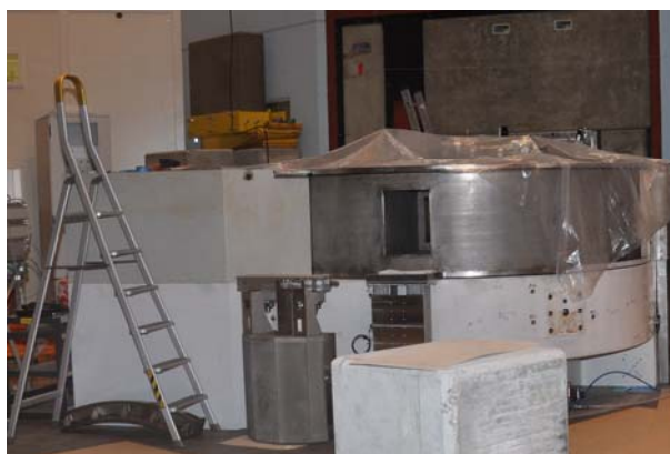
Figure 8: The secondary spectrometer of EIGER in place on the high-precision granite (left) and the lower part of the base monochromator shielding with turning unit.
