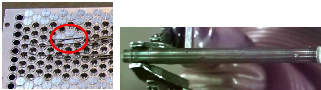
Figure 1: Left: Rod array of SINQ Target 5: The Zr-clad rods are clearly distinguished (flat covers) from the steel-clad ones: three peripheral rows and an assembly of 4 rods in the centre (encircled). Right: Visual inspection of one of the 4 central Zr-clad rods after 2 years of irradiation in the SINQ target.
