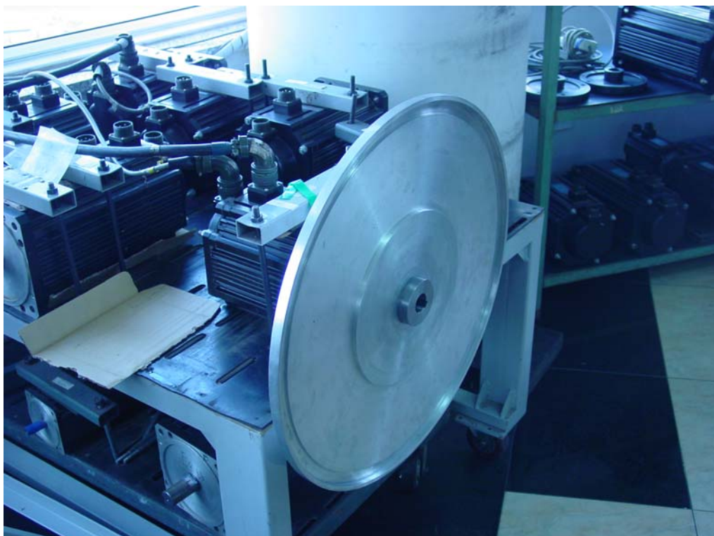
Figure 3. The prototype bandwidth-limiting chopper under development for the CPHS project.
