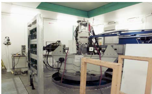
Fig. 3 SMARTS load frame that is capable of applying forces up to 250 kN to massive samples up to 1500 kg. A companion furnace/cryogenic capability provides temperature environments from liquid N 2 to 1700 C.
