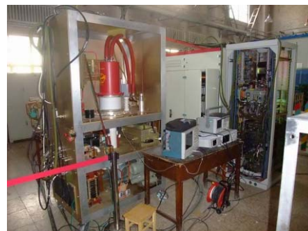
Figure 12 A 500kW RF power source has been developed
