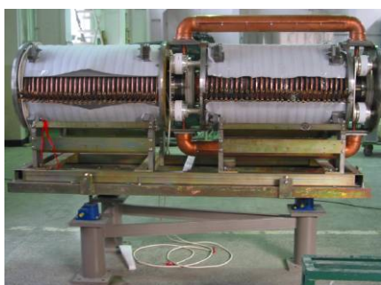
Figure 11 The prototype of the ferrite loaded RF cavity.
