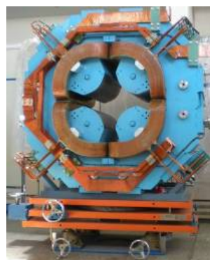
Figure 8 The prototype quadrupole magnet
