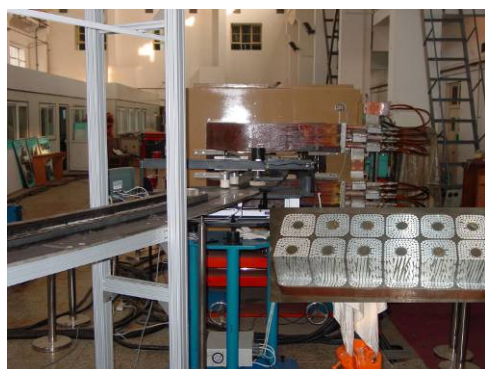
Figure 7 The prototype dipole magnet of stranded coil and the measurement system
