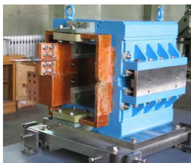
Figure13 The prototype injection bump magnet.
